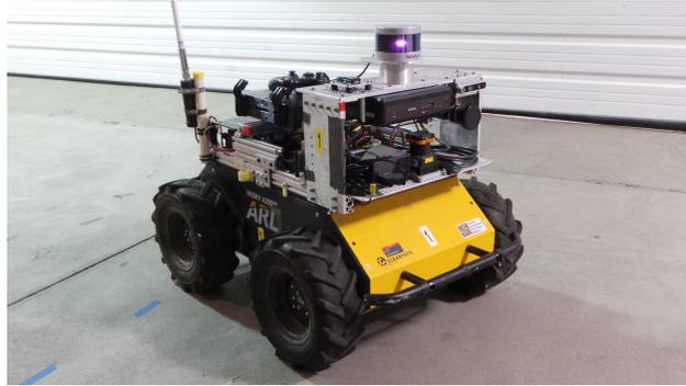
**Figure 15.** Clearpath Husky robot used for system integration and evaluation.
