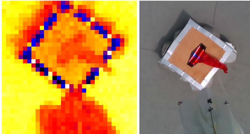
**Figure 7.** Example of the thermal detection of a ground fire. Left, thermal image. Right, same view from the visual camera.
