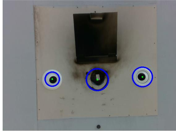
**Figure 9.** Output of the Hole Detector. The facade fire is not active but its central fire ring is detected with the RGB-D camera. The additional holes to simulate wind gusts are the same size and hence also detected.
