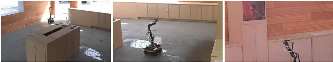
**Figure 8.** UGV navigating towards the target (left), performing heat source detection (center), and abating the detected heat (right).
