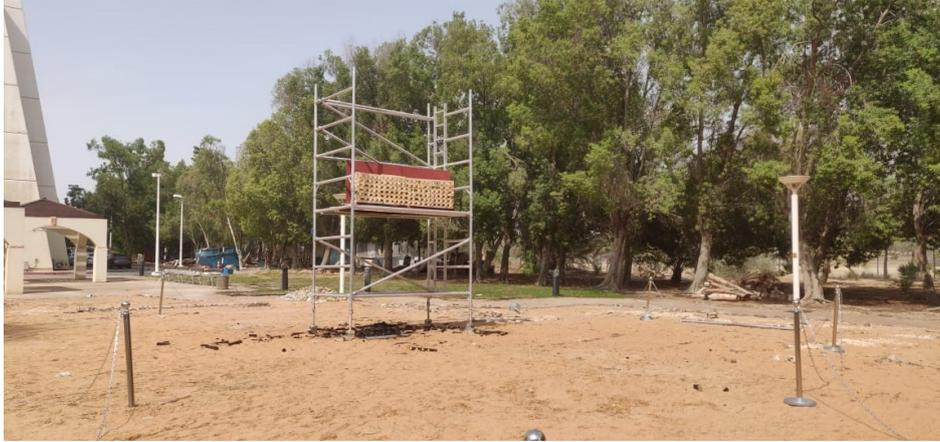
**Figure 14.** Firefighting testing facility with a wood crib of size 10A\* raised at three metres. A metallic back-plate is used to improve mechanical stability, and improve radar readings stability.
