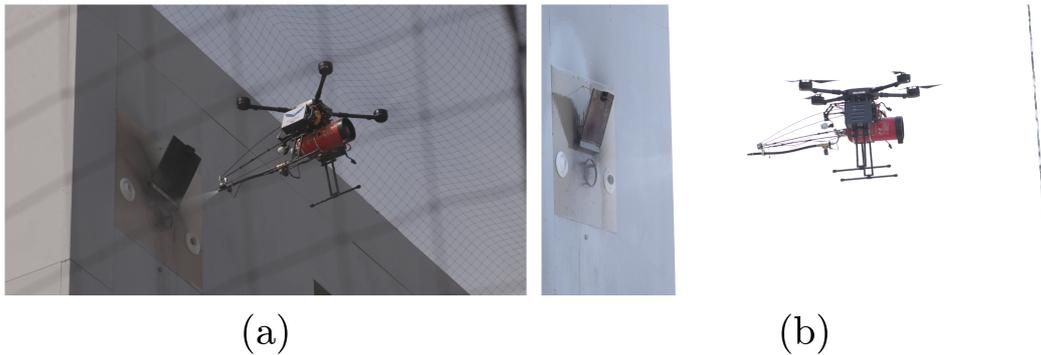
**Figure 16.** Photos of the firefighting UAV targeting façade fires during MBZIRC2020. The fire in (a) is located at the second floor of the mock building used for Challenge 3. The fire in (b) is being targeted from a distance of about two meters.
