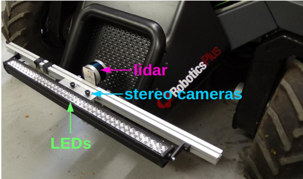
**Figure 6.** Parts of the spray boom height controller hardware on the front of the mobile robot platform.
