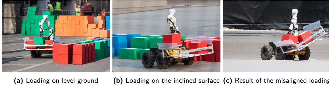
**Figure 21.** Loading bricks into the cargo bay using the manipulator arm. On level ground, the robot was able to fill the cargo bay as intended. However, during the competition, the bricks were positioned on an inclined ramp, which ran through the center of the arena. In such a case, the bricks were not being lowered into the cargo bay along a vertical line. As a result of the misalignment, the bricks could not have been stored with the expected level of precision.
