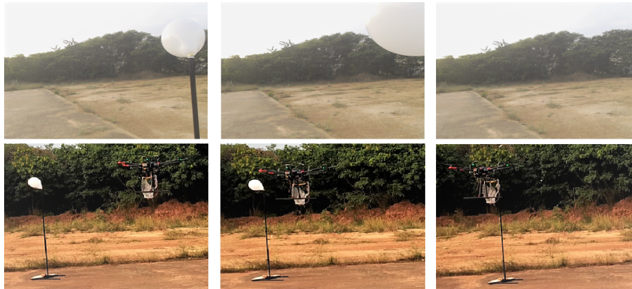
Figure 32. Balloon-popping experiment from the UAV camera (top) and third person (bottom). From left: detection, approaching and popping. The experiments were carried out using a white balloon.
