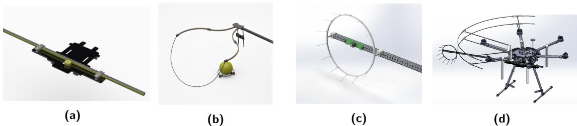
Figure 28. The relevant design components of the manipulation mechanism are (a) The rack and pinion mechanism (linear actuation) with its mount (b) The end effector to grab ball (c) The end effector for popping balloons (d) The manipulator along with propeller guards.
