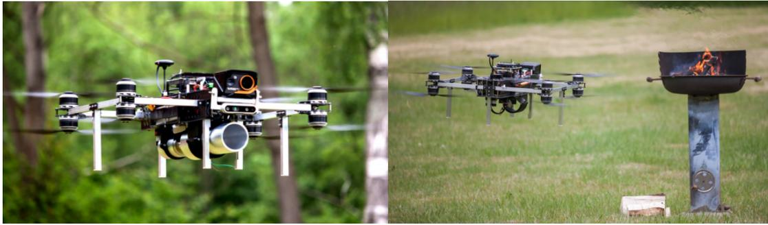
**Figure 21.** Our working prototype of a firefighting UAV designed for using gas-based extinguishing capsule launcher - an evolution of the system developed for the MBZIRC 2020 competition.
