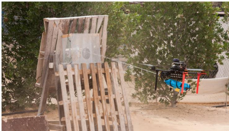
**Figure 15.** Preliminary test in the desert with only fire extinguishing on a fire analogue.
