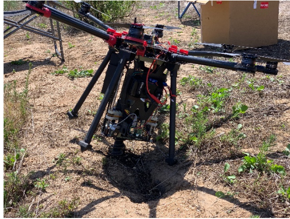
Figure 18. False positive: Poor slope identification resulting in unsuccessful sensor implantation
