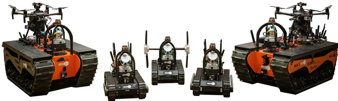
**Figure 23.** The Urban Circuit robot fleet consisted of two BIA5 ATRs each carrying an Emesent Hovermap UAV, and three Superdroid LT2-F platforms.
