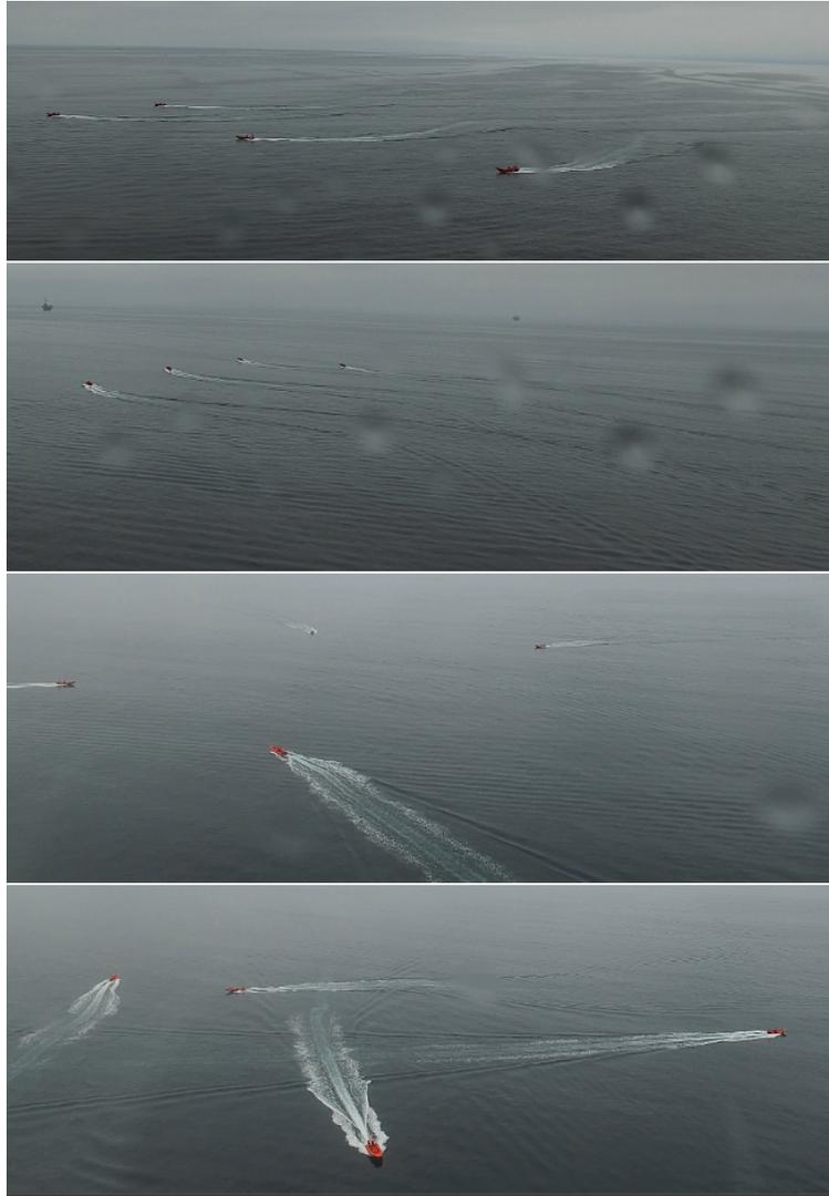
**Figure 17.** A 2019 test filmed from a remote-controlled quadrotor. The boats are conducting two tests at high speed, a weaving formation transit, and a four-way crossing. The boats are under completely autonomous control and are uncrewed.
