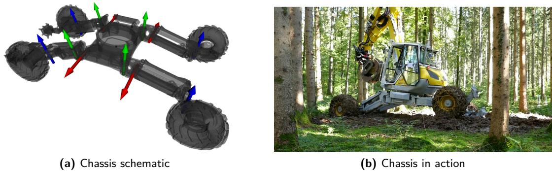
**Figure 14.** *Left:* Illustration of the HEAP's chassis. The cabin and the arm are not shown for the sake of clarity. Steering joints axes are shown with blue arrows, flexion joint axes with red, and abduction joint axes with green color arrows. The path following controller actuates the steering joints while the HBC actuates the flexion joints. Abductions joints are not used. *Right:* Chassis control system overcoming a stump during the deployment.
