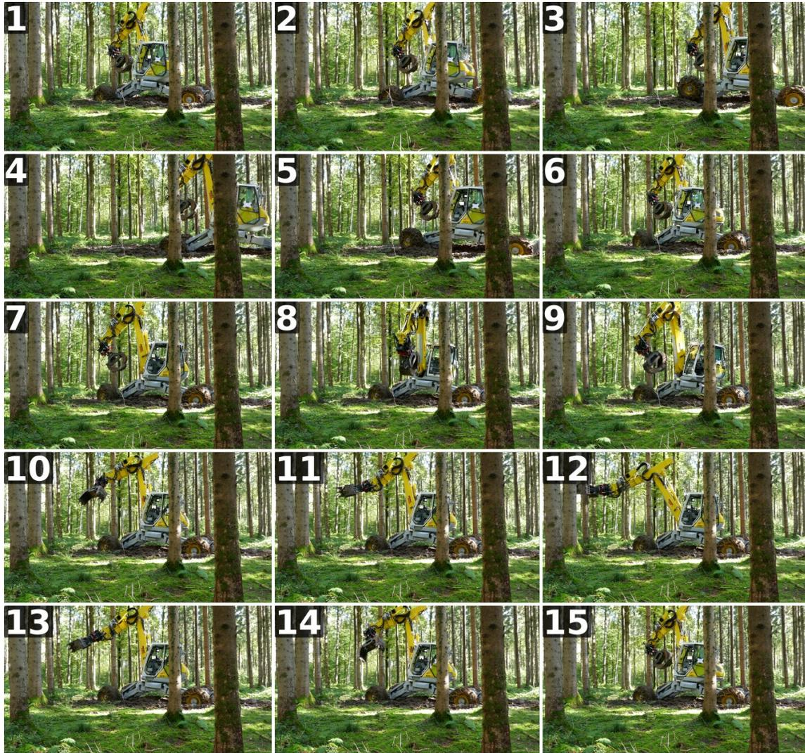
**Figure 40.** Snapshots of an operational cycle between grabbing two trees. HEAP re-positioning the base close to the tree (snapshots 1-6) followed by scanning the environment and building a local map (snapshots 7-9). Finally, HEAP grabs the tree by extending the arm (snapshots 10-12) and retracting it (snapshots 13-15). After retracting the arm, the harvester is ready to grab the next tree and whole cycle repeats.
