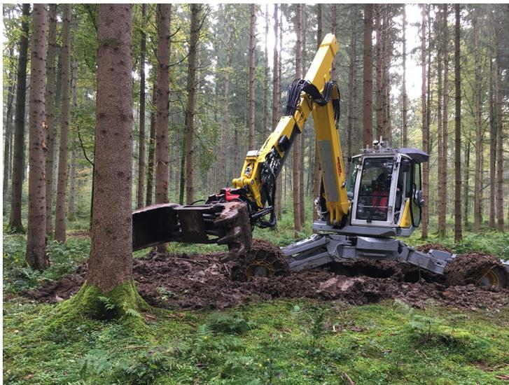
**Figure 3.** Legged excavator navigating to a tree and performing a grab. Human is in the cabin for safety reasons.
