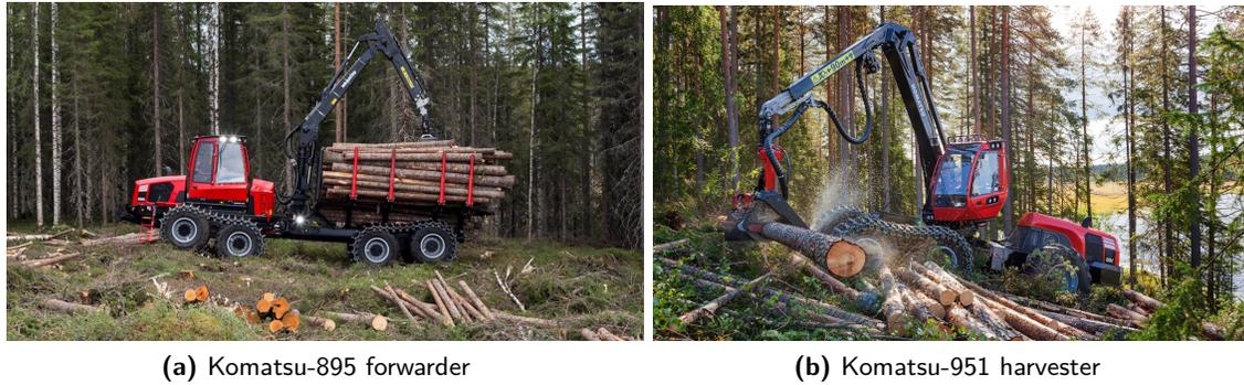
**Figure 1.** Different machines are typically used in modern forestry operations. They all have operator cabins to increase the comfort level in a possibly wet and muddy forest environment. Images were taken from [Komatsu Corporation, 2019].
