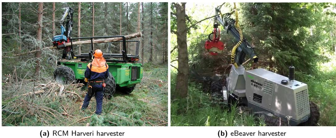
**Figure 2.** Smaller harvesters that are typically used for thinning operations. They do not have a cabin for the operator and are remotely controlled within the operator's line of sight. Images taken from [Jukka Hämeekoski, 2016] and [Magnus Gustavsson, 2016].
