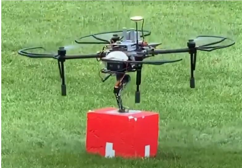
**Figure 11.** The UAV in contact point with a red block.
